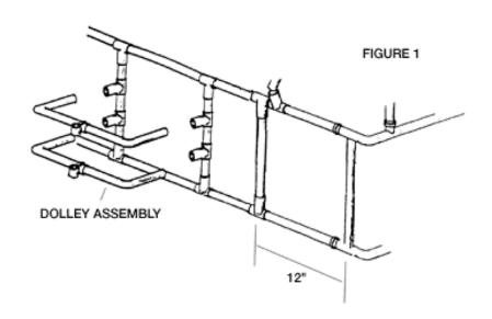
1. Assemble the Back Assembly using two 190" tubes and four 32" tubes and "T" fittings as shown in Figure 1. Place two 32" tubes approximately 12" from each end and center the tubes for the dolley assembly. Please refer to Figure 1.
