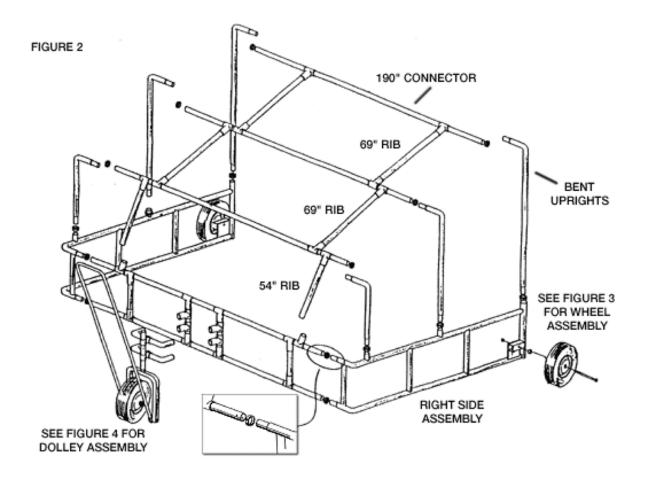
2. Position the Back Assembly, Right Side Assembly and Left Side Assembly as shown in Figure 2. Slide a Locking Collar on each end of the Back Assembly and slip the Side Assemblies in place.
