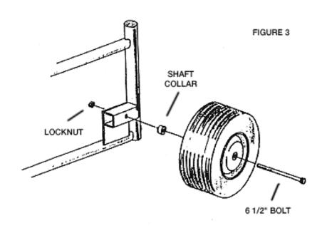
3. With the lower portion of the Backstop now assembled, install the Wheels by inserting an 6 1/2" Hex Bolt in through the Wheel. Slide a Shaft Collar on the bolt and insert through the Wheel Mounting Bracket on Side Assembly as shown below. Screw the Locknut onto the Bolt until the Bolt tip is flush with the Locknut. Lock down the Shaft Collar against the Mounting Bracket. Refer to Figure 3.
