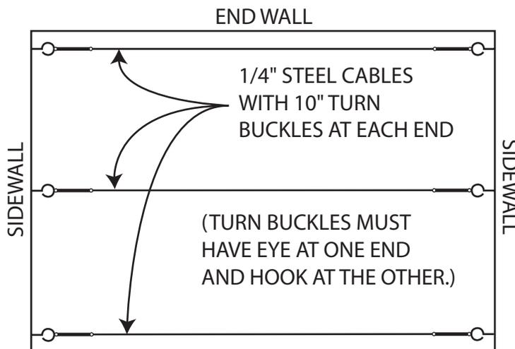
3. Attach the vertical cables this way:
