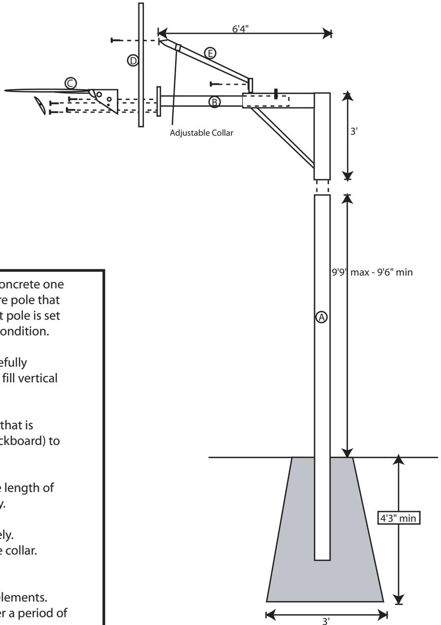
1. Set pole to depth shown on the illustration. With concrete one foot below the pole. Make sure when setting square pole that flat side of pole is square with playing area and that pole is set straight. Concrete installation may vary upon soil condition.
